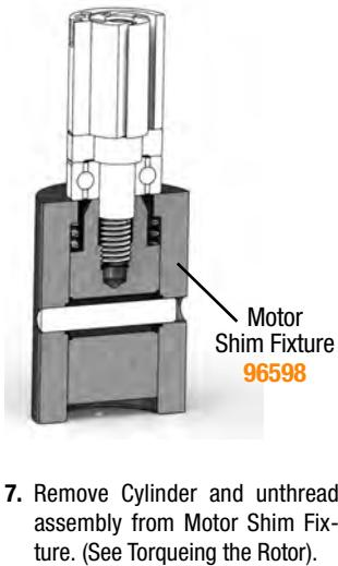
7. Remove Cylinder and unthread assembly from Motor Shim Fixture. (See Torqueing the Rotor).
