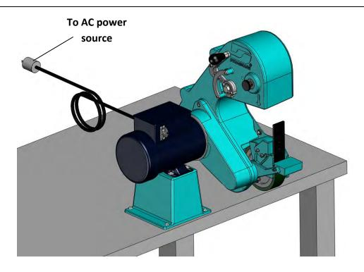
With Power off, install desired abrasive belt on machine. Begin by releasing tension on assembly to allow for clearance and belt to slip on to three wheel assembly as shown.
