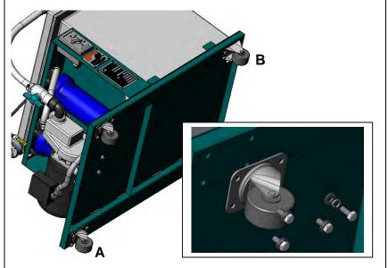
After removing your system from the pallet, install casters provided to the bottom of the assembly as shown. Qty 2 rigid and Qty 2 swivel casters are provided for mounting. Swivel casters (A) are mounted at the pump end of the assembly. Rigid casters (B) are to be mounted at sump/tank end of assembly, as shown in detail.
