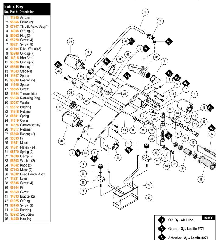
Shaded part numbers represent 14334 Tension Wheel Assembly.
