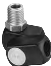
Dynaswivel® Swivels 360° at two locations which allows an air hose to drop straight to the floor, no matter how the tool is held. • 94300 1/4" NPT
