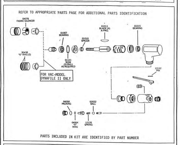
IMPORTANT: THE REGULAR MAINTENANCE OF ANY AIR TOOL WILL CONTRIBUTE TO GREATER EFFICIENCY OF TOOL AND WILL PROLONG TOOL LIFE. THIS KIT CONTAINS REPLACEMENT PARTS WHICH ARE MOST SUSCEPTIBLE TO WEAR. AN AIR TOOL MAY WEAR DIFFERENTLY ACCORDING TO THE APPLICATION AND OPERATOR. IT IS, THEREFORE, RECOMMENDED THAT WHILE THE TOOL IS DISASSEMBLED, ALL OTHER PARTS MOT INCLUDED IN THIS KIT BE EXAMINED FOR EXCESSIVE WEAR AND BE REPLACED AS REQUIRED.
