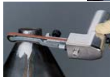
Slack of abrasive belt is used to efficiently polish radiused area.
