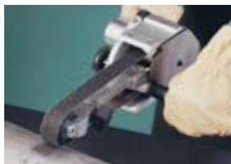
Model 11475 is ideal for grinding circumferential welds.
