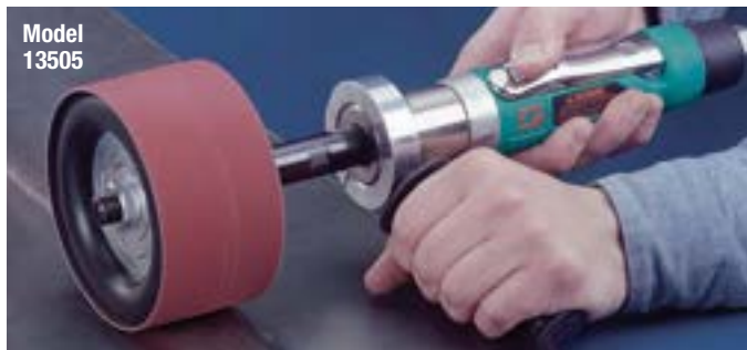
13505 Dynastraight® powers optional 94472 Dynacushion® pneumatic wheel.
